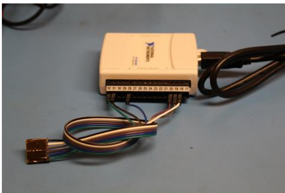
Figure 7: NI USB-6501 USB-to-SPI Interface Device - USB AB 2.0 Cable + Custom Cable Assembly Attached
