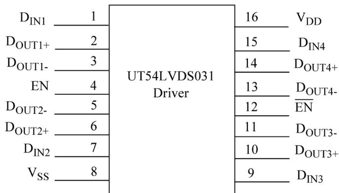
Figure 2. UT54LVDS031 Pinout
