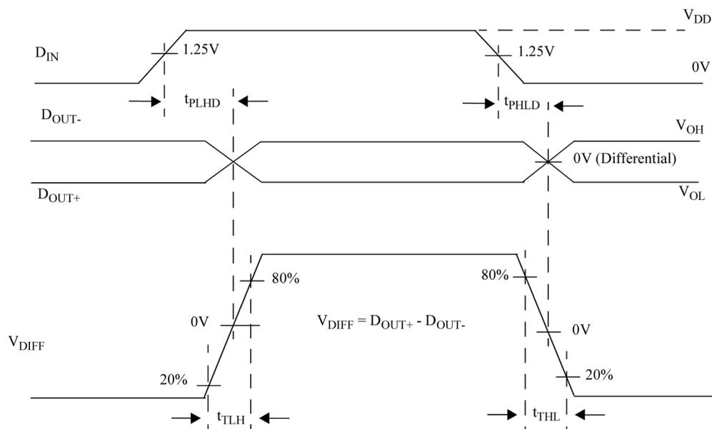
Figure 7. Driver Propagation Delay and Transition Time Waveforms
