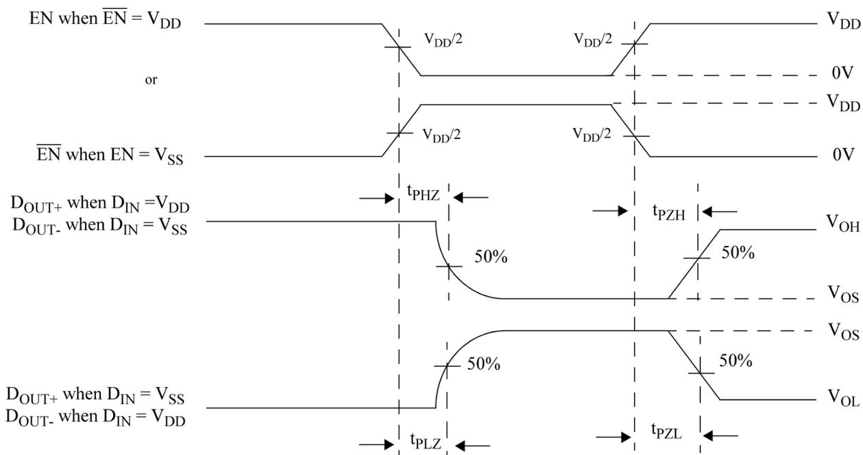
Figure 8. Driver Three-State Delay Waveform or Equivalent Circuit
